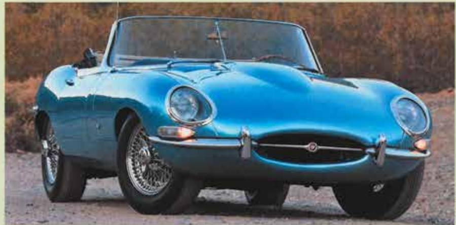
Series 1 Open Two-Seater and Fixed-Head Coupe have glass-covered headlamps until 1967.
