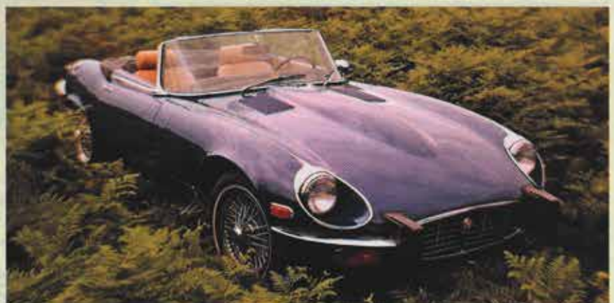
Series 3 cars have eggcrate grilles, flared wheel arches, and three styles of impact bumpers on U.S.-spec cars.
