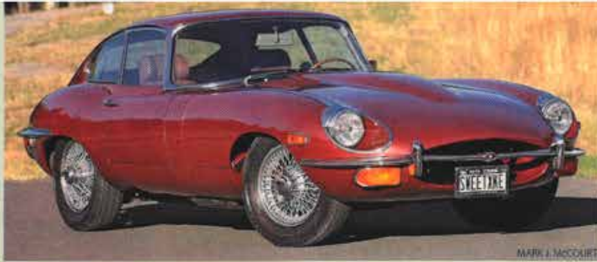
Series 2 cars have larger air inlets, uncovered headlamps set forward in their scoops, and larger parking and taillamps moved below the bumpers.
