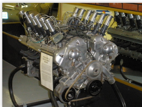
Dual overhead cam, fuel injected v12 designed for the mid-engine xj13
